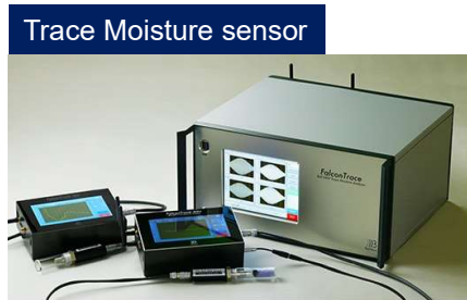
Figure 1. Trace moisture sensors by ball SAW technology
