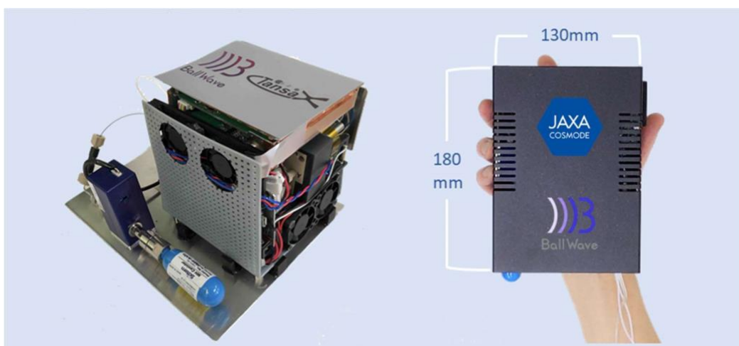
Figure 1. Gas chromatograph for space probe applications (left) Gas chromatograph for terrestrial applications (right)
