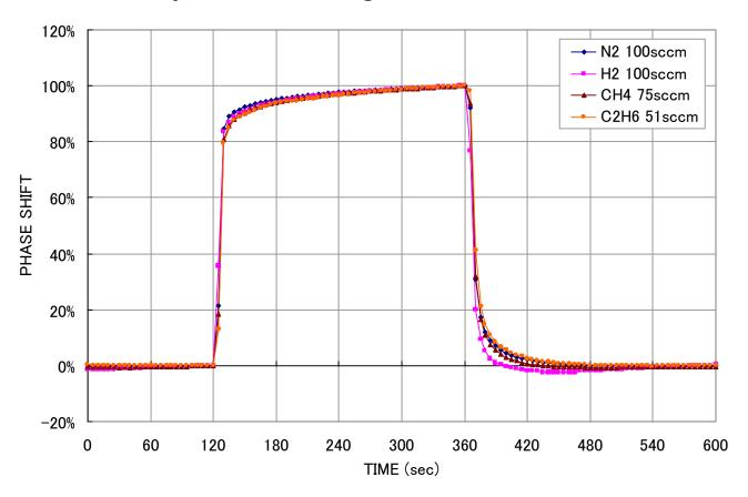
Transient Characteristics @ 1,800ppm H<sub>2</sub>O Injection
