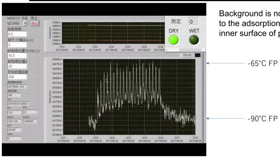
Background is not an artifact but is due to the adsorption of moisture on the inner surface of piping.
